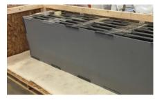
Skids and crates are custom built to ship panels to every project. Panels are numbered, packed and shipped in sequence based on the predetermined plan for installation.
